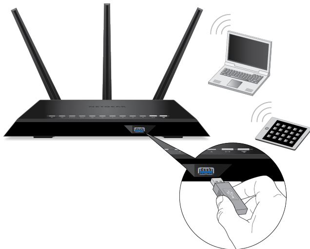
Figure 6. One USB 3.0 port is located on the front panel of the router
